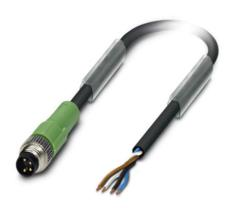
Sensor/actuator cable, 4-pos., PUR halogen-free black, straight M8 plug on free conductor end, cable length: 3 m
